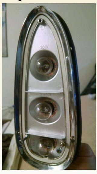
OEM 9" 101 series tail light assembly restored. New tail light to body mounting gasket, a new lens gasket, all new SS hardware, and all new light bulbs. The lens is useable, though not pristine. One may notice that the signal portion of the lens isn't amber, it's red. It's the original stock lens.
