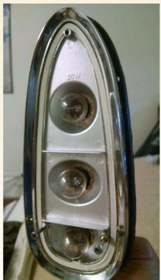
OEM 9" 101 series tail light assembly restored. New tail light to body mounting gasket, a new lens gasket, all new SS hardware, and all new light bulbs. The lens is useable, though not pristine. One may notice that the signal portion of the lens isn't amber, it's red. It's the original stock lens.
